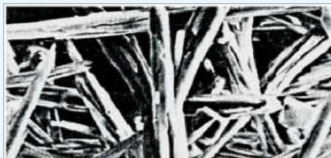
Picture 11: Lime dust deposits
