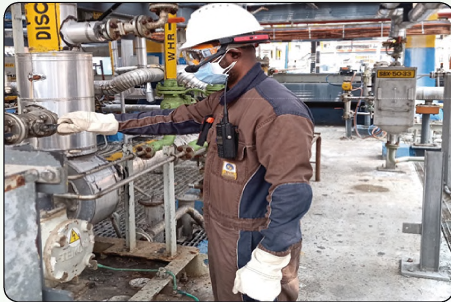
Image 2:- Use of helmet mounted 'REAL WEAR' device for on the spot two way communication in Acrylates unit.
