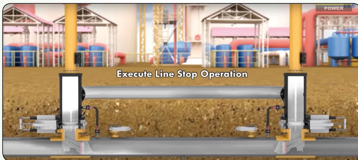
Fig 1: Representative schematic of "Line stop" Operation
