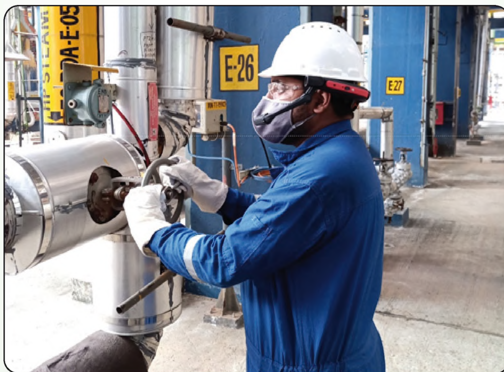
Image 1:- Use of helmet mounted 'REAL WEAR' device for on the spot two way communication in Acrylic acid unit
