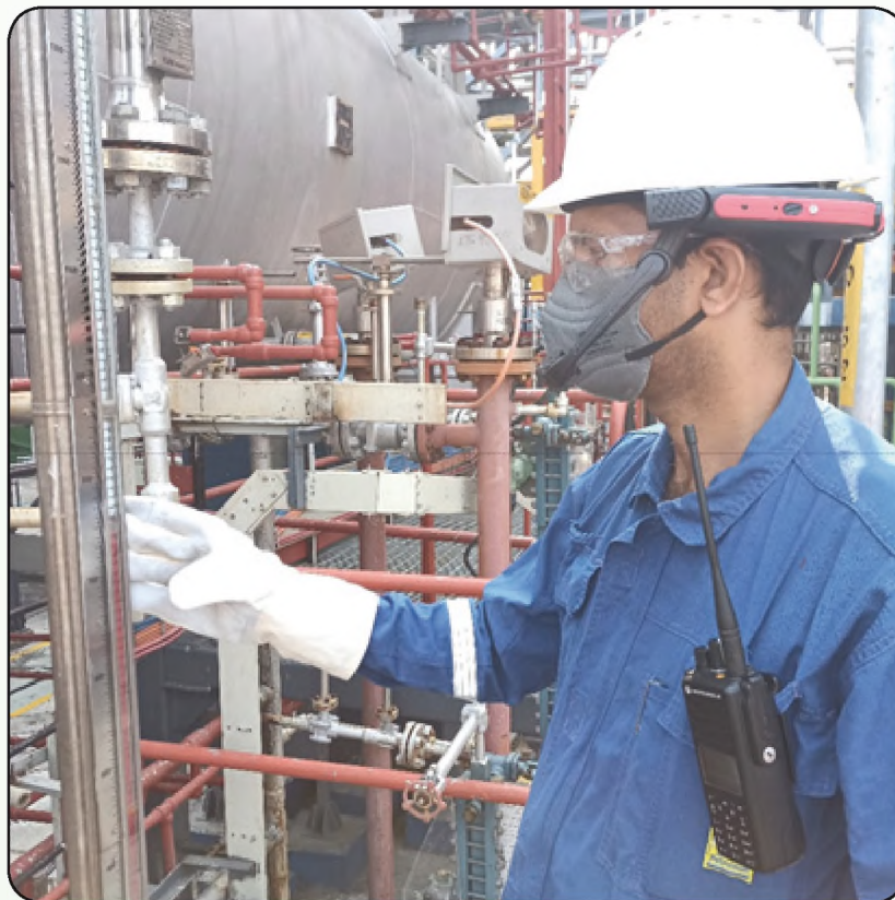
Image 3:- Use of helmet mounted 'REAL WEAR' device for on the spot two way communication in Oxo alcohol unit.
