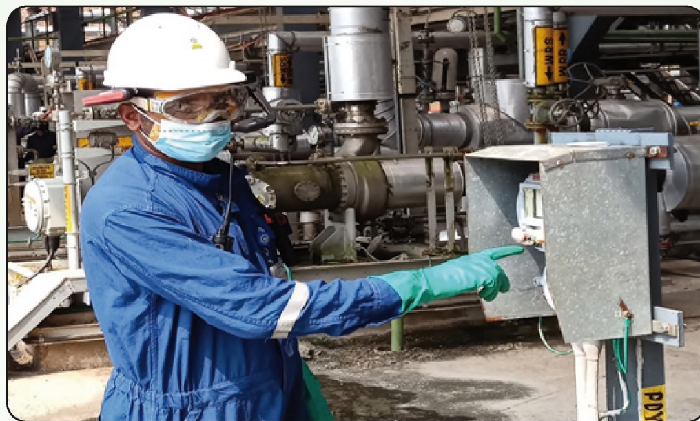
Image 4:- Use of helmet mounted 'REAL WEAR' device for on the spot two way communication in Offsites and utilities unit
