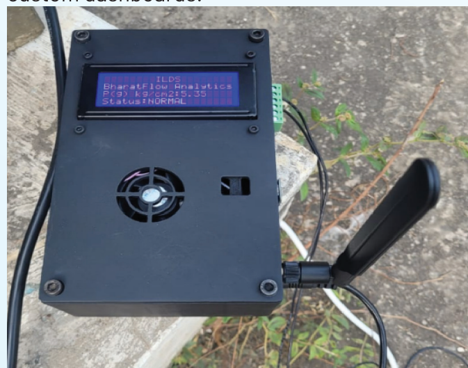
Fig.-9. IIoT Edge Device for faster data collection and cloud integration
