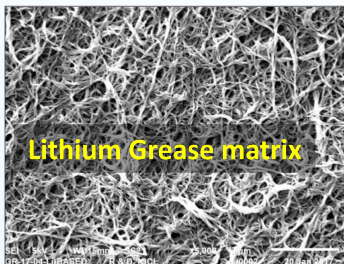
Fig. 1: SEM of Lithium grease
