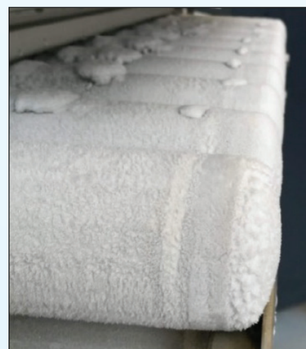
Fig. -4: Storage module which is frozen because of fast (leak) flows.
