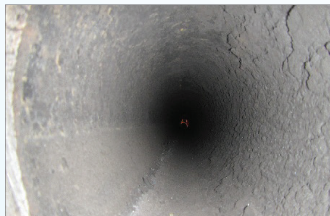
Fig. -11: Coking inside Tubes
