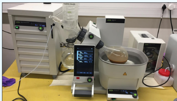
Fig 5. Rotavapor equipment for vacuum Distillation Model BUCHI R300
