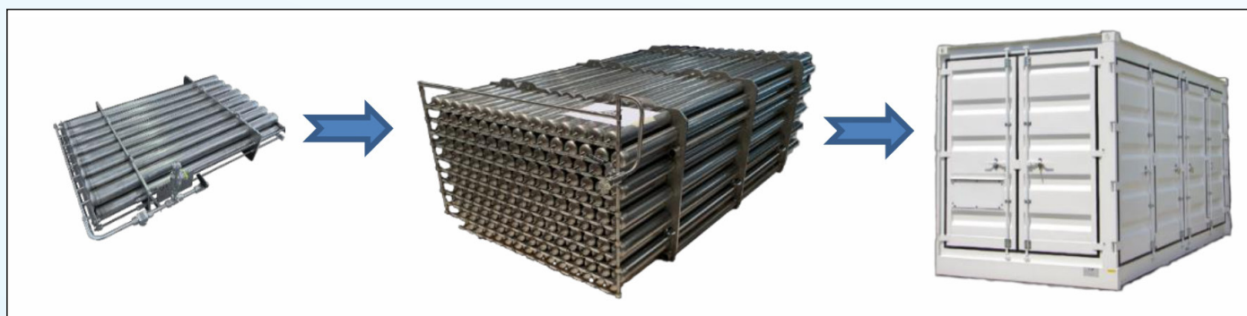
Fig. -5: Scalability of MH based Hydrogen storage in parallel Tubular structures
