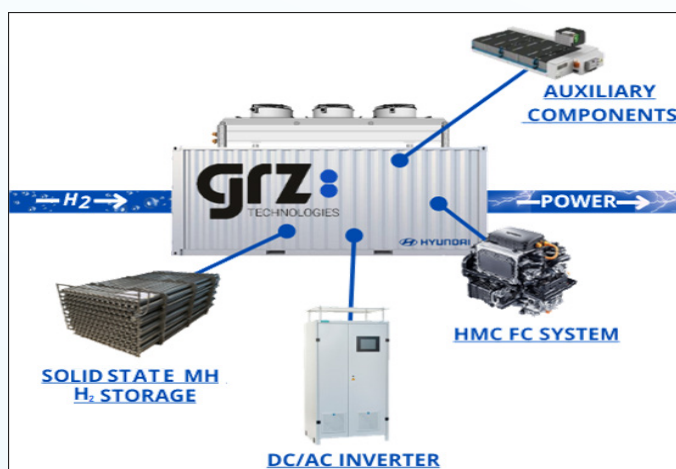
Fig. -6: Dash Power combining MH Solid Hydrogen Storage, Fuel cell, DC/AC inverter and Aux components.
