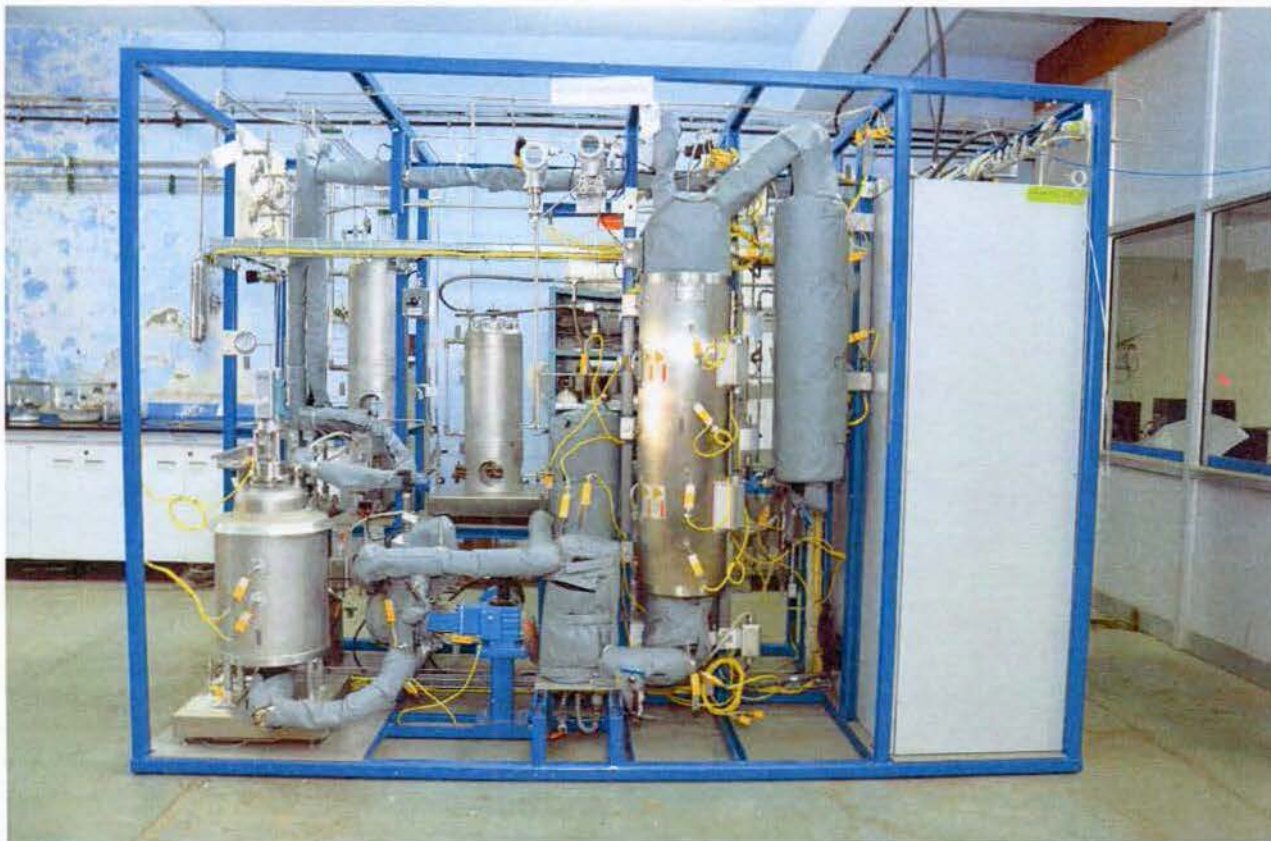
Slurry Hydrocracker pilot facility at CSIR-IIP
